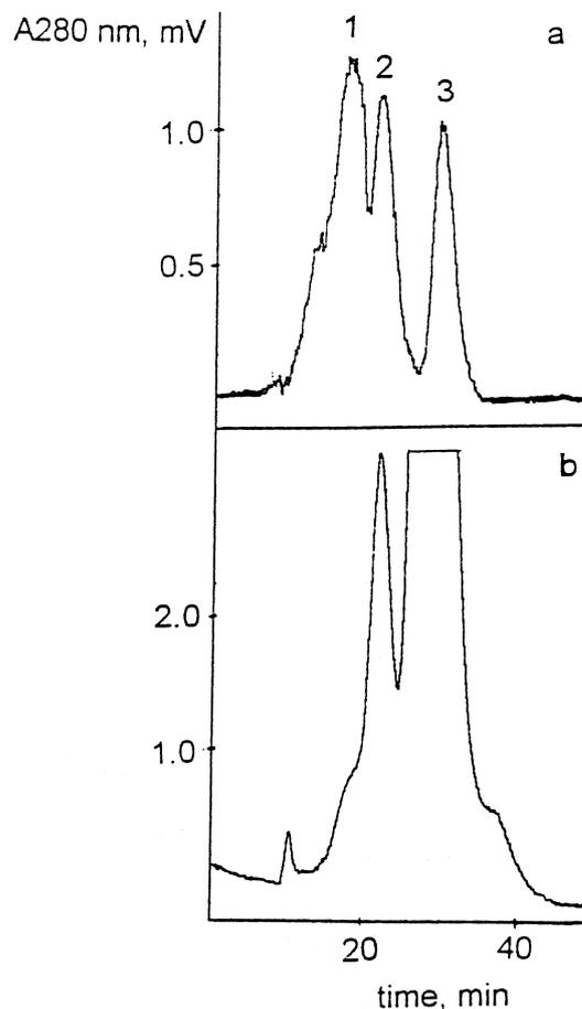
Fig. 3. Chromatogram of the 18–20 min fraction of peak 2. Conditions as in Fig. 3. Injection volume, 100 µl (a), 125 µl (b); sample buffer, 417 mM DTT, 4.2% (w/v) SDS and 16% (v/v) 2-mercaptoethanol (b). Peaks: 1=HBsAg dimer and 2=HBsAg monomer.
