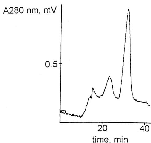
Fig. 5. Chromatogram of fivefold-concentrated fraction corresponding to peak 1 remaining after reduction with 417 mM DTT, 4.2% (w/v) SDS and 16% (v/v) 2-mercaptoethanol. Conditions as in Fig. 1. Injection volume, 50  $\mu$ l.
