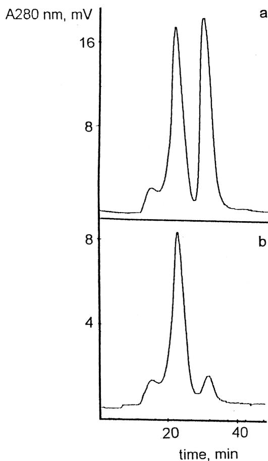
Fig. 4. Chromatogram of reduced HBsAg before (a) and after (b) filtration. Conditions as in Fig. 1. Injection volume, 50  $\mu$ l; sample buffer, 417 mM DTT, 4.2% (w/v) SDS and 16% (v/v) 2-mercaptoethanol. Reduction procedure as described in Section 2.
