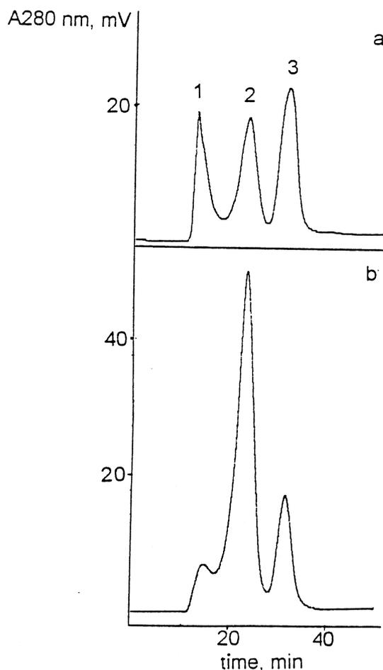
Fig. 1. Chromatogram of reduced HBsAg. Conditions: TSK G4000 SW (600×7.5 mm I.D.); eluent, 0.3% SDS, 0.1 M Tris-HCl, pH 7.0; flow-rate, 0.9 ml min<sup>-1</sup>; detection, UV at 280 nm; injection volume, 75 μl; sample buffer, 0.3 M Tris-HCl, 10% (w/v) SDS and 25% (v/v) 2-mercaptoethanol (a), 417 mM DTT, 4.2% (w/v) SDS and 16% (v/v) 2-mercaptoethanol (b). Peaks: 1=HBsAg oligomer, 2=HBsAg monomer and 3=low molecular mass compounds.
